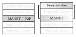
c) Integrated MP2P d) Cross Layered MP2P
